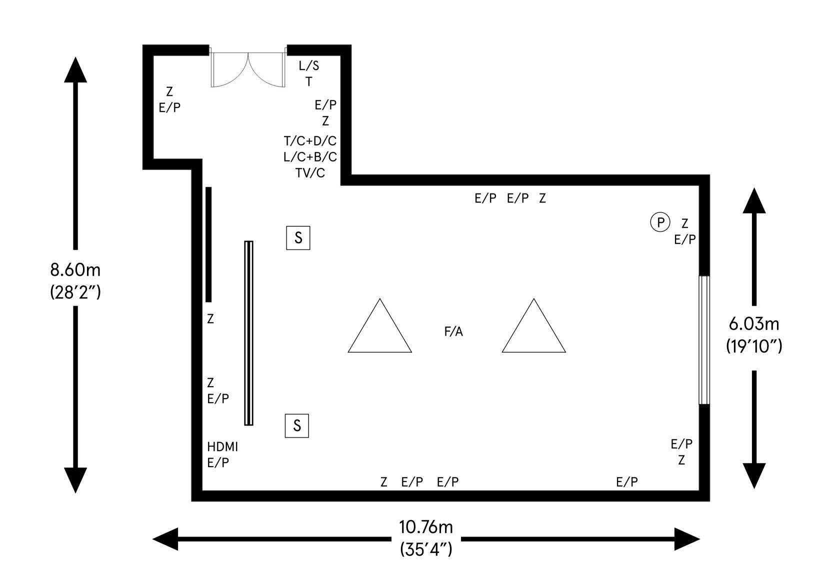
Key: 13 Amp Sockets Speaker Ethernet Port Chandelier TV/C Television Control Phone Line Light Switch Audio/Video Socket L/C Lighting Control HDMI HDMI Input B/C Blinds Control Wall Mounted Television D/C Digital Screen Control Dropdown Projector Screen **Emergency Test**
