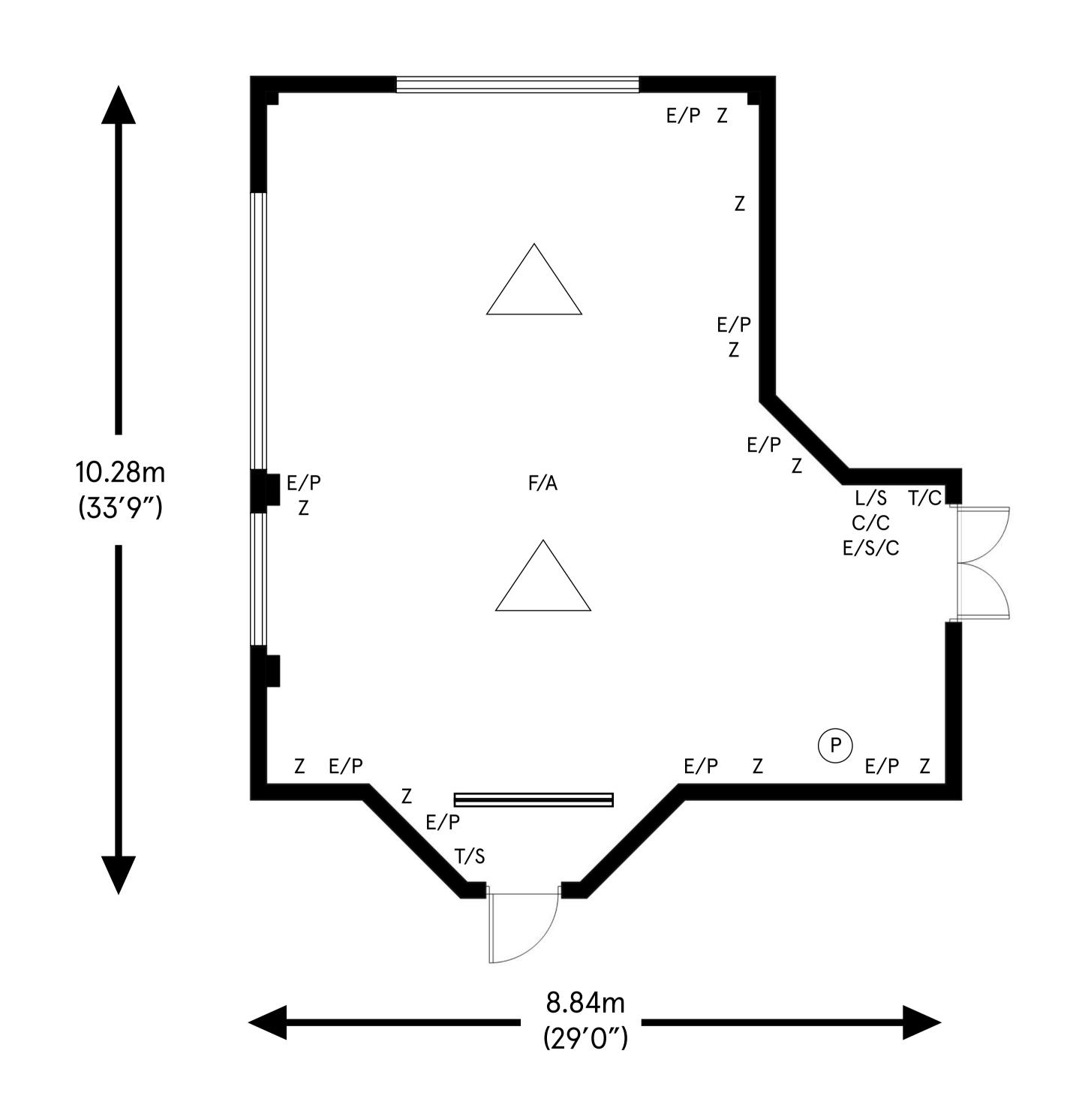
Key:Z13 Amp Sockets△ChandelierE/PEthernet PortT/CTemperature Control(P)Phone LineT/STV SocketL/SLight switch Panel→Drop Down Projector ScreenC/CCurtain Control→Drop Down Projector ScreenE/S/CElectric Screen Control
